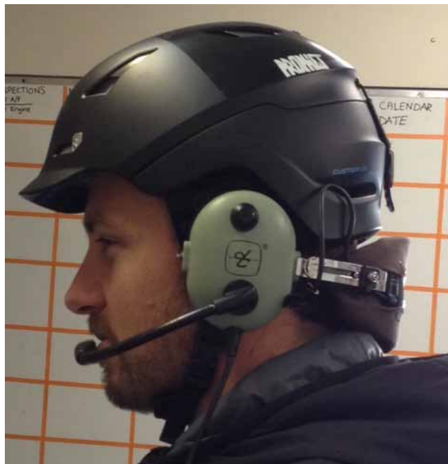
Headset modification for use with helmet. Photo courtesy of John Furneaux
